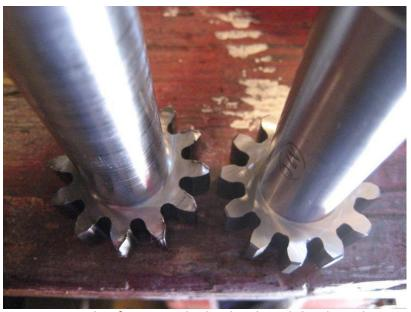
any impression. The photo' shows an example of one supplied unhardened that lasted less than 1,000 miles before the backlash became alarmingly obvious. The photo also shows the correct shape of teeth for comparison.
